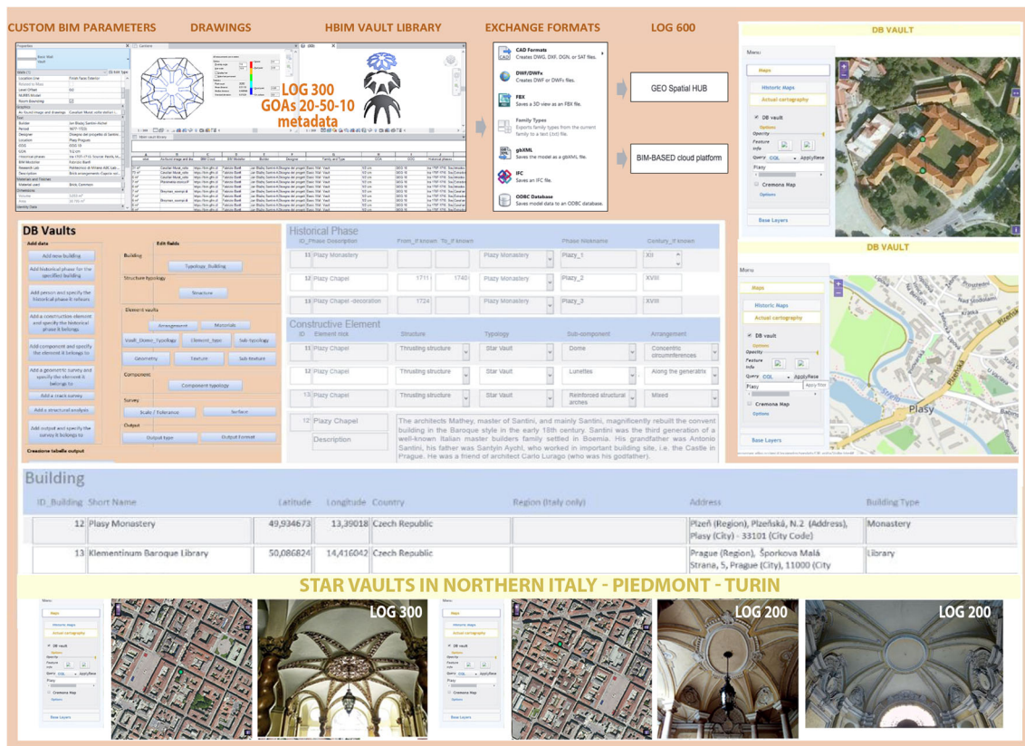
Fig. 14 The HBIM vault library and its exchange formats for LOG 600 through the Geospatial Hub and the BIM-based cloud platform (upper). The GeopanAPP was implemented within the Geospatial Virtual Hub with the Vault GEODB and linked HBIM object libraries. Queries based
