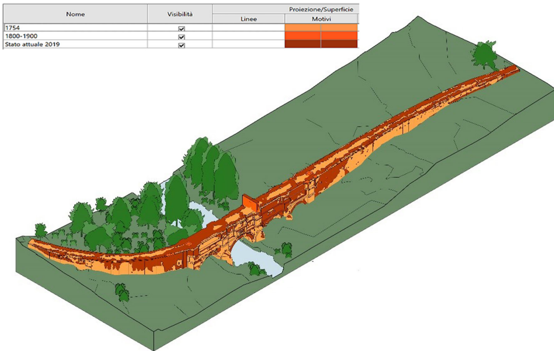
Fig. 9 Time sequence of the bridge, obtained filtering the construction phases in the HBIM model
