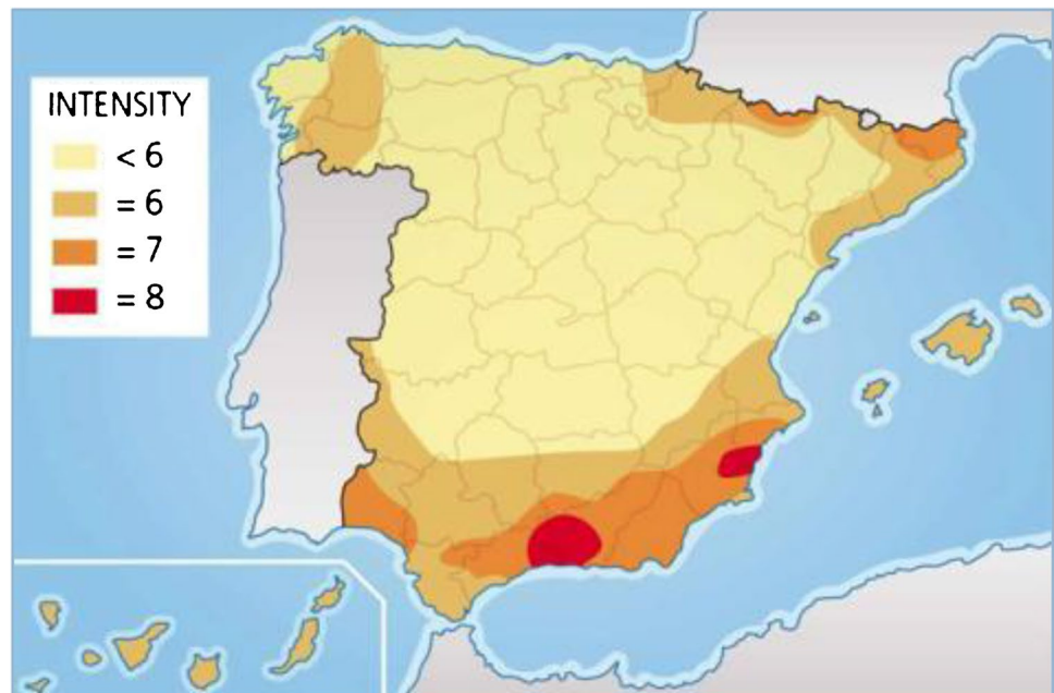
Fig. 2 Spain seismic hazard as EMS intensity for a 475 years return period (IGN-UPM 2013)
