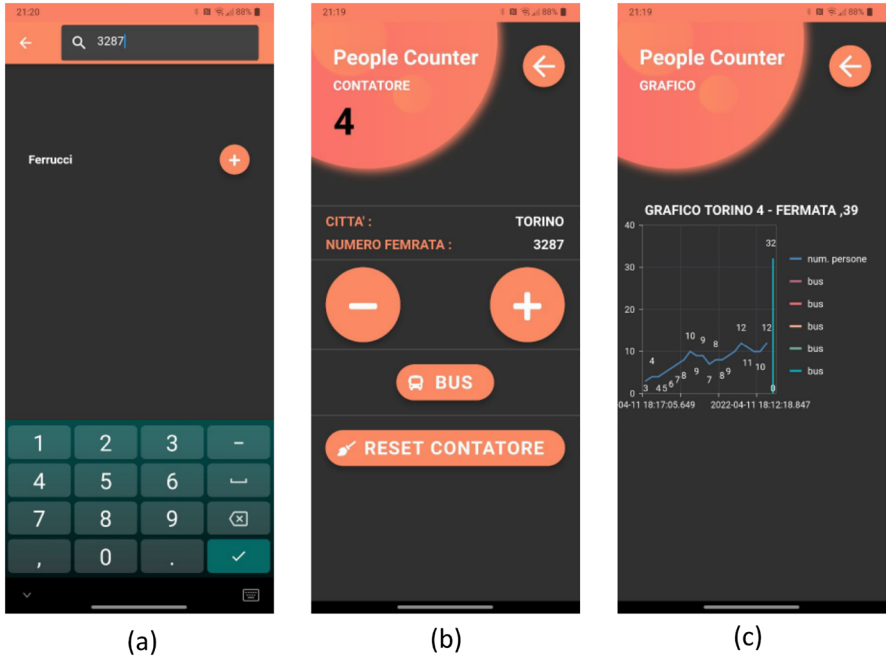
Fig. 2 People Counter app screenshots: a Search screen, b Count screen, c Plot screen
