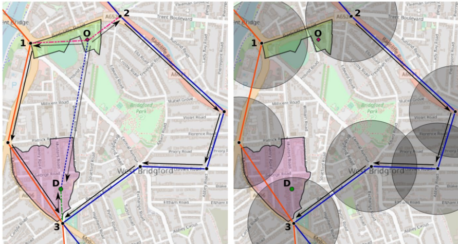
Fig. 1 Example of the impact of different trip representations on trip options. Assumed is a trip between two zone centroids O and D . Two PuT routes can be used: “orange” over nodes 1 and 3, and “blue” over nodes 2 and 3. In a zone-based approach (left), travellers can choose from three options: a walk from O to 1, ride on route “orange” to 3, and walk from 3 to D ; b walk from O to 2, ride on route “blue” to 3, walk on from 3 to D ; c use the direct walking connection from O to D . In the node-based approach (right) the trip is assigned to nodes based on their catchment areas (grey circles). Travellers have only one option: travelling on route “blue” from 2 to 3. Walking is not considered. (The zones displayed in the figure were taken from the sets of zones described in Sect. 4.1. The map underlying the image is taken from https://www.openstreetmap.org .)
