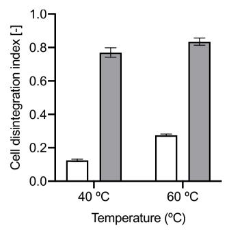
**Fig. 6** Cell disintegration index at different stages of blanching of carrots blanched in water at 85 °C (unfilled bars) and by ohmic-PEF heating at 1330 V/cm and 100 Hz (grey bars). Adapted from Astráin-Redín et al. [18]
