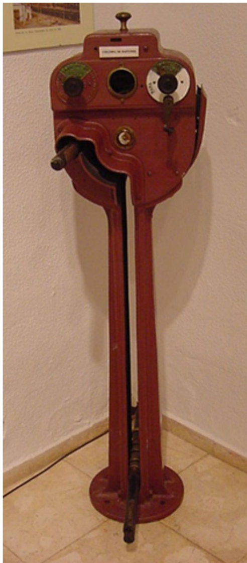
Fig. 12 Manual switch stand used on the railway
