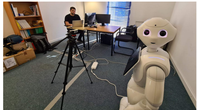
Fig. 1 The lab settings, including the robot Pepper (SoftBank Robotics) in front of a web camera, while the experimenter in the back is controlling the robot using the Wizard of Oz technique
