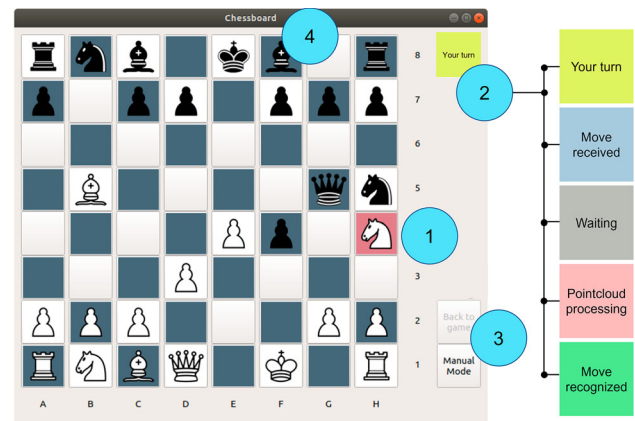
Fig. 4 User interface chessboard window. The game situation is represented on the screen. When the user moves the input device (touchpad, mouse, or joystick) the currently selected square is highlighted in light red (label 1). When selecting a move, the start and end square will be highlighted in dark red and yellow, respectively (not shown in this Figure), waiting for the user to confirm. The user is constantly informed of the application status (label 2). Errors in the move recognition can be manually corrected enabling the “Manual Mode” (label 3). Clicking the button opens a pop-up window with tools to cancel, add or replace pieces on the virtual chessboard. A similar pop-up window opens in case of promotion, i.e. when a pawn reaches the last rank on the opposite side (label 4)
