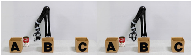
Fig. 3 Human-like feedback design. During the response delay of 10s, the robot taps the desk with its fingers
