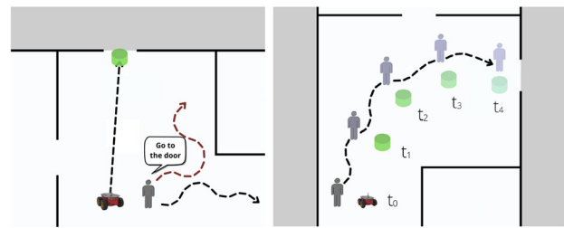
Fig. 5 Task versus interaction. The main difference between task and interaction sources of rewards is their spatial definition. Sources whose location is independent of any team member's movement actions are considered task sources, even if they are generated through direct interaction (e.g. the verbal command stated in the left image: "go to the door"). Interaction rewards are those whose spatial definition is generated in one of the team members' reference. Typical examples would be side-by-side navigation, which is depicted in the right image. Notice the goal moves according to the agent's actions and it would change if they took another path
