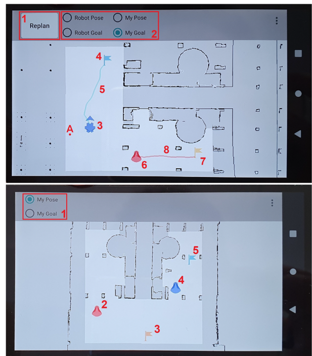
Fig. 16 Mobile App main screen. Top : Screenshot of an ongoing human–robot collaborative search where the human has used every available functionality. 1) Replan button. 2) Input data selection menu. 3) Robot's current position. 4) Human's desired goal for the robot. 5) Path calculated by the robot. 6) Human's current position. 7) Human's intended goal. 8) Path calculated for the human. Bottom : Execution using a simplified version of the interface for human–human collaborative search experiments. 1) Input data selection menu. 2) Human's current position. 3) Human's intended goal. 4) Human's partner position. 5) Human's partner intended goal. (Color figure online)
