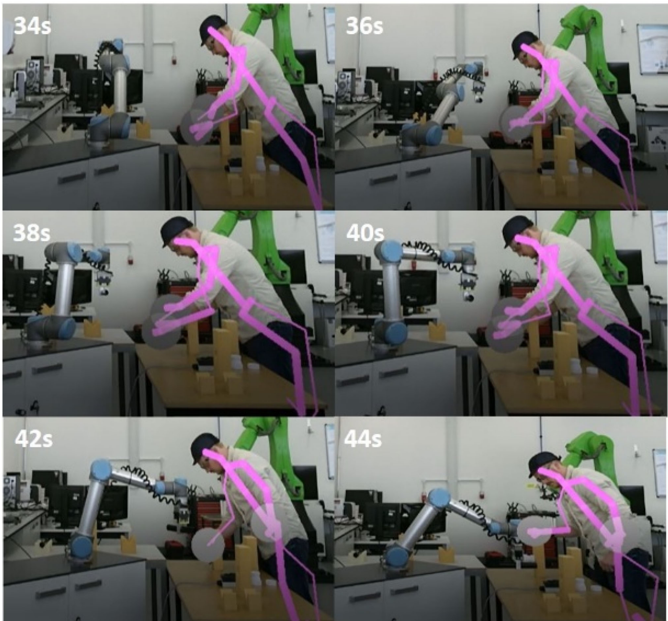
Fig. 2 A time-lapse of the experiment, where the UR5 avoids the participant before moving to the holding position with the pipe. The algorithm is activated on the 38 s mark, in this case avoiding the head as it has the closest proximity
