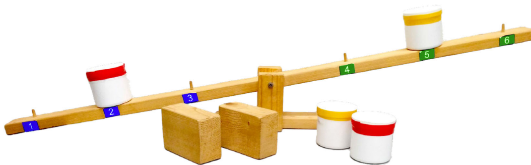
Fig. 2 The wooden balance with several differently weighted pots that can be placed over the pins and wooden blocks that can be placed underneath the balance
