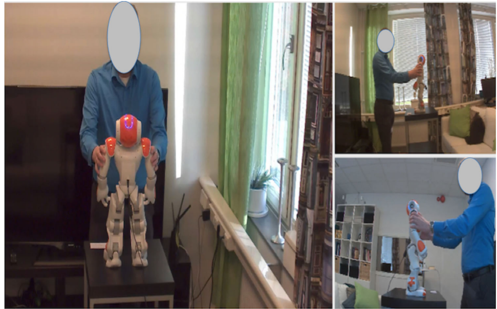
Fig. 1 Experimental set-up where the participant interacts with the Nao in the Usability Lab. This participant interacts with the Nao by touching left and right arms to convey a particular emotion. Camera shots are displayed and analyzed using the ELAN annotation tool
