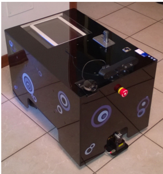
Fig. 6 The KuBo robot, built upon a youBot KUKA platform is used for the experiments
