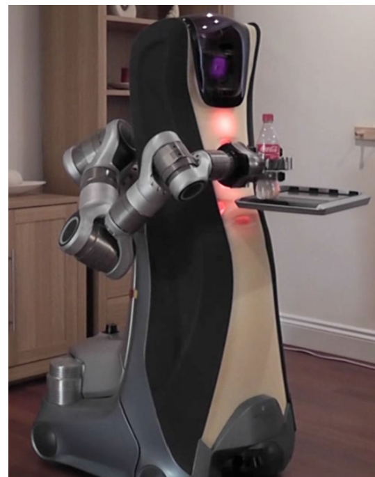
Fig. 5 Care-O-bot ® 3 placing a bottle on its tray while its LED display panel is showing red colour. (Color figure online)
