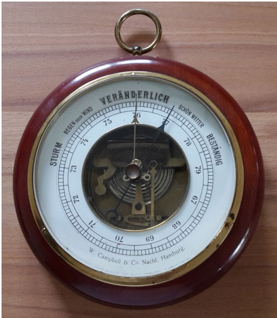
Fig. 6 Aneroid barometer. The metallic membrane in the background is deformed by air pressure (structural information) and turns the pointer in the foreground over a scale divided in units of mm Hg (symbolic information). Written number symbols serve for easier counting of the units. Private photo
