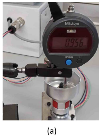
Fig. 19 a Setup for measuring the earing height evolution b equipment to measure the total cup height
