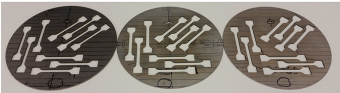
Fig. 5 Tensile Samples cut from blanks showing orientation
