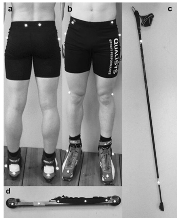
Fig. 3 Placement of the 30×12-mm reflective markers on the athletes' joint centres and anatomical locations (a, b), poles (c) and roller skis (d), with identical placement on lateral aspects of both the left and right sides. Anatomical locations included anterior and posterior superior iliac spines, femoral greater trochanter and lateral epicondyles, malleolus, heel and toe centre
