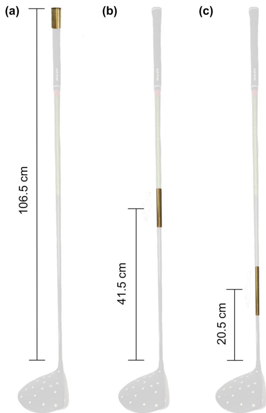
Fig. 1 The locations of the additional mass used to vary the MOI of the three club conditions: a low MOI; b mid MOI; c high MOI
