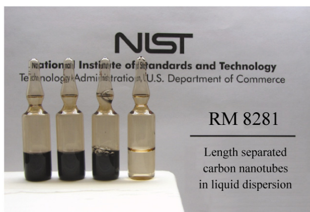
Figure 1 Photograph of (left to right) the Long, Medium, and Short length-sorted nanotube dispersions after ampouling and gamma irradiation. The blank reference solution containing only 1% sodium deoxycholate is displayed to the right. The dispersions display a uniform appearance with no visible settling or aggregate formation. The irradiation process itself induces a yellowing of the initially clear glass ampoules
