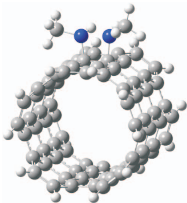
Figure 12 Calculated structure of 5,5 SWNT \text{C}_{80}\text{H}_{20} fragment with two N -methyl amino ( -\text{NH}-\text{CH}_3 ) groups (1,2-addition)
