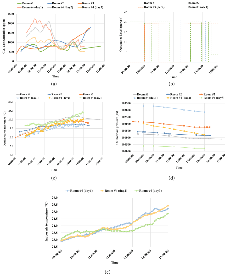
Fig. 3 (a) CO 2 concentration measurements, (b) occupancy level profiles, (c) outdoor air temperatures, (d) outdoor air pressures, and (e) indoor temperatures
