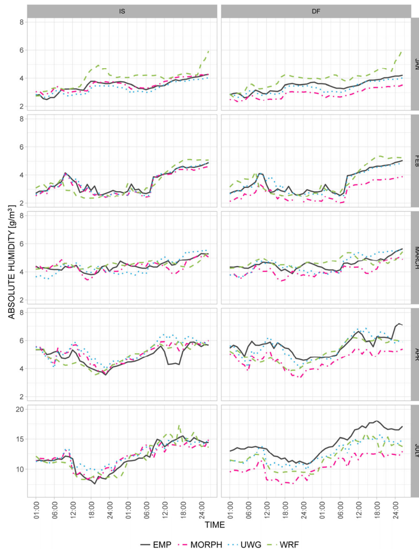
Fig. 2 Hourly distribution of absolute humidity from WRF, UWG and morphing approach compared to empirically obtained data (EMP) for urban areas IS (left) and DF (right)
