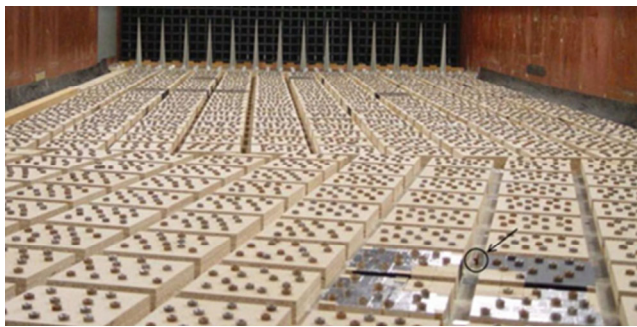
Fig. 21 Wind tunnel set-up of building array with indication of source position (Garbero et al. 2010; reproduced with permission ©Springer)
