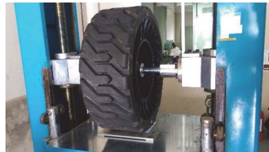
Figure 3. Vertical stiffness testing of TWEEL.
