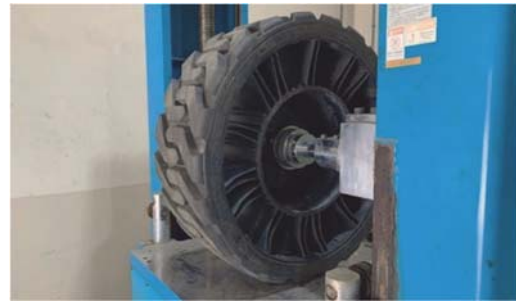
Figure 12. Stiffness testing on the authentic TWEEL with the reduced-spoke case n = 15b .
