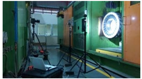
Figure 2. Setting up of high speed video camera to record NPT's spoke deformation during rotation.
