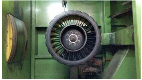
Figure 1. Drum testing of NPT, Tweel 12N16.5 SSL ALL TERRAIN by Michelin.
