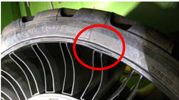
Figure 18. Separation at spoke-shear band interface.
