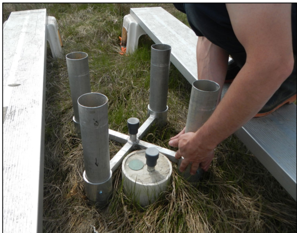
Fig. 3 Shallow RSET installation nested within deep RSET station. Shown here before pipes were trimmed flush to receiver completing the installation. This placement differs from protocols (Lynch et al. 2015) because the authors wanted to maximize overlap between deep RSET and shallow RSET measurements, facilitate logistics of reading both stations, and minimize the chance of trampling if the benchmarks were more offset
