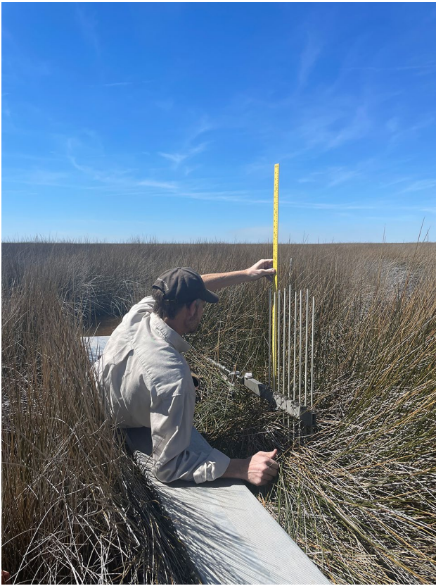
Fig. 2 Surface elevation table (SET) monitoring apparatus. The level SET arm extends above the benchmark and nine equally spaced pins are placed through holes in the arm. The height of the pins above the SET arm are measured for long-term trends in elevation. Photo courtesy of Michelle Moorman, USFWS
