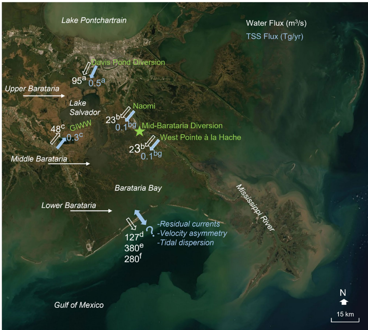
Fig. 3 Water and sediment fluxes in Barataria Bay inferred from observations and modeling. Solid white arrows denote geographical regions. Solid blue arrows and hollow white arrows represent water fluxes and sediment fluxes, respectively. Legends in green indicate inflow sites (GIWW, Gulf Intracoastal Waterway). The site of the proposed future mid-Barataria sediment diversion is represented by a green star symbol. Mean water discharge at Naomi from 2006 to 2019 was used to infer mean discharge for both Naomi and West Pointe à
