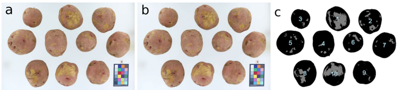
Fig. 3 Original image (a, 6000×4000 pixels) versus resized image (b, 1500×1000 pixels) and indexed tubers with skinned area shown in gray (c)
