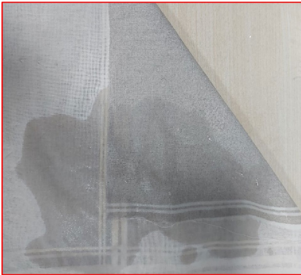
Fig. 2 The picture of back and face surface of D0 (untreated) applied fabric during the water absorbency test
