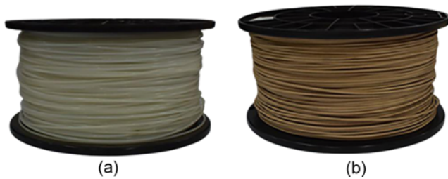
Figure 14. Filaments for 3D printing: (a) PLA and (b) BF-PP-PLA. Adapted with permission from [103], Copyright 2018, Society of Plastics Engineers.
