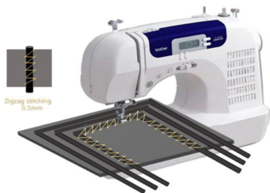
Figure 4. Fabrication of SMA textile actuator with zigzag stitching.
