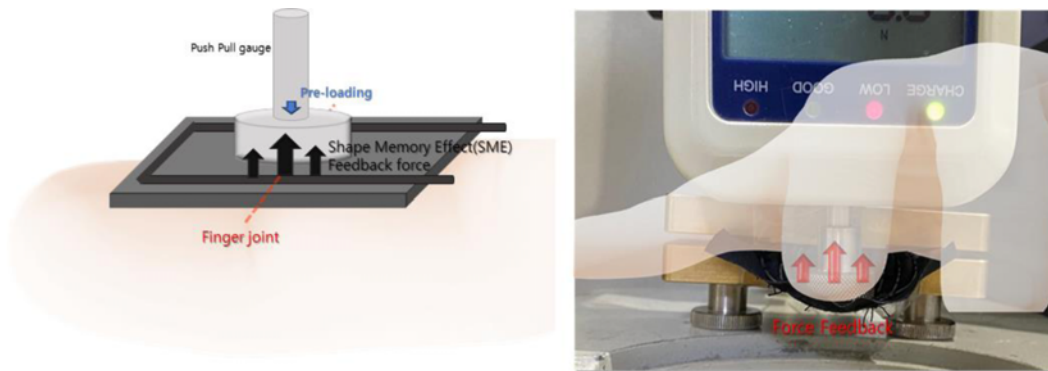
Figure 7. Measuring force feedback with SMA textile actuator with push-pull gauge.
