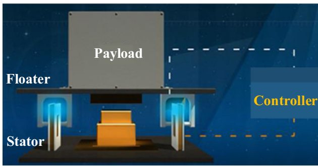
Fig. 1 Principle of microgravity active vibration isolation system
