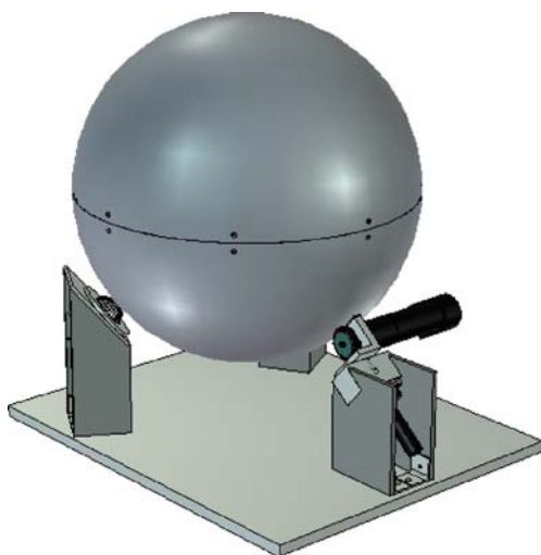
Fig. 1 Ball RPM. The ball RPM is supported on two freely rotating contact points. The third contact point is a wheel connected to a motor that drives the rotation of the large sphere. The orientation of this motor and drive wheel can be varied by a second motor. The combined control of these motors allows a free walk path over the sphere, resulting in a continuously change in orientation of the sphere with its suspended sample system
