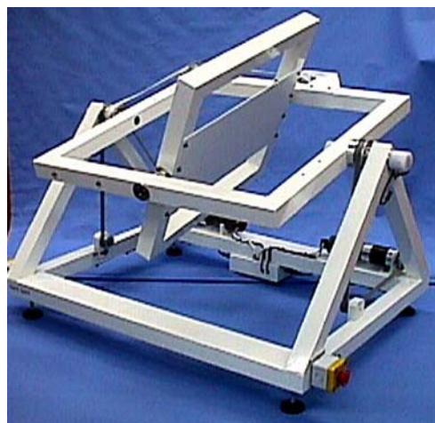
Fig. 2 RPM with two independently driven perpendicular frames
