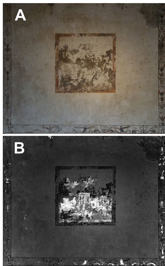
Fig. 11 An example of degraded painting in Grande Criptoportico . Visible image (A) and conventional VIL NIR image (B)
