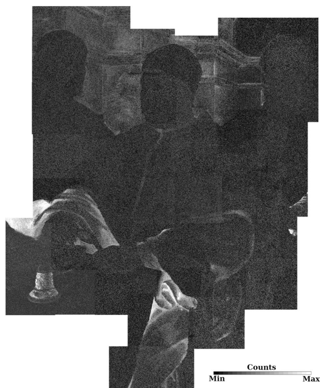
Fig. 2 The elemental distribution of Bi L \alpha line. The visible image of the painting and the complete characterisation of its palette can be found in Mazzinghi et al. (2022)
