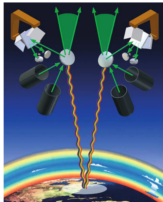
Fig. 3 Schematic of the CLARREO interferometer. There are two independent instruments boresighted on the same region of the surface. There are four independent black bodies ; a minimum of one would suffice
