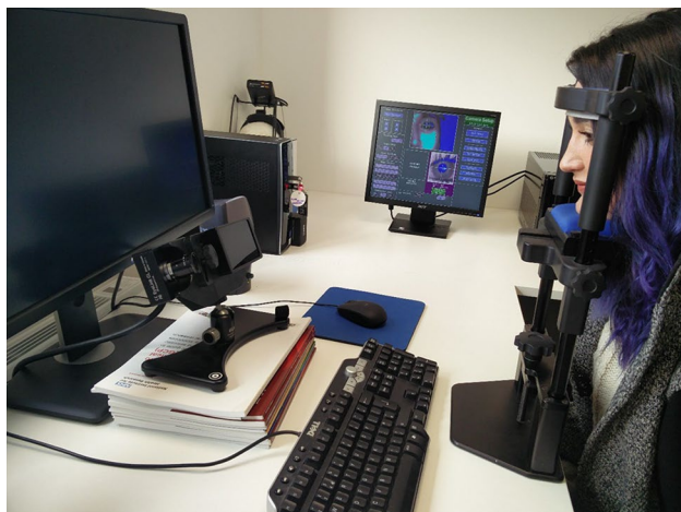
Fig. 1 Experimental setup showing the EyeLink 1000 Plus apparatus and a prototypical participant looking at the screen
