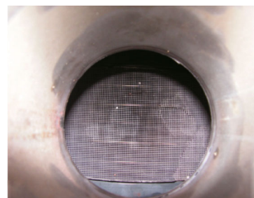
(c) Converter inlet top view through 4" exhaust pipe with charging tungsten wires spaced above the converter (high-voltage power supply off)
