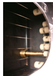
(f) Charger wires-electrode-ceramic insulator assembly view
