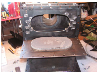
(b) Electrically stimulated catalytic converter housing
