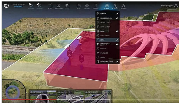
Fig. 11 View of the Břežno tunnel portal via Accur8vision visualization software - setting up detection zones (Hexagon 2023a)
