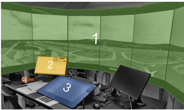
Fig. 6 The RTC simulator used for the evaluations, including annotations for the different components. 1: Animated 3D Tower View of the runway. 2: Radar display for the airspace surrounding the airport. 3: Touch screen for interacting with the electronic flight strips. 4: Headphones used to listen to the sonification
