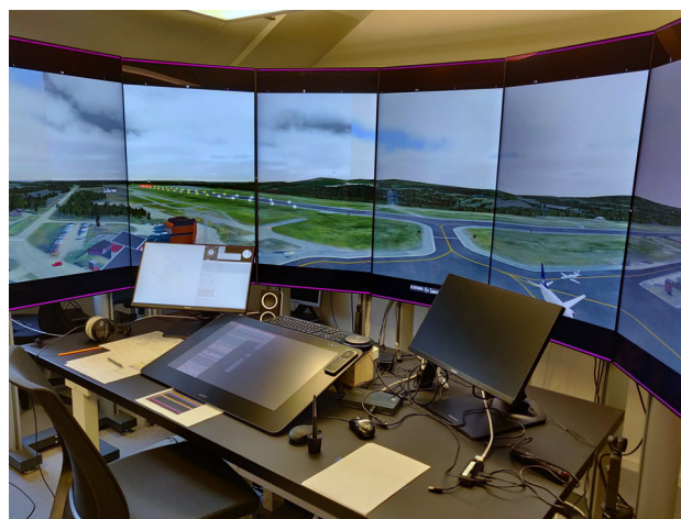
Fig. 1 The remote tower center (RTC) simulator where the sonification was integrated and evaluated
