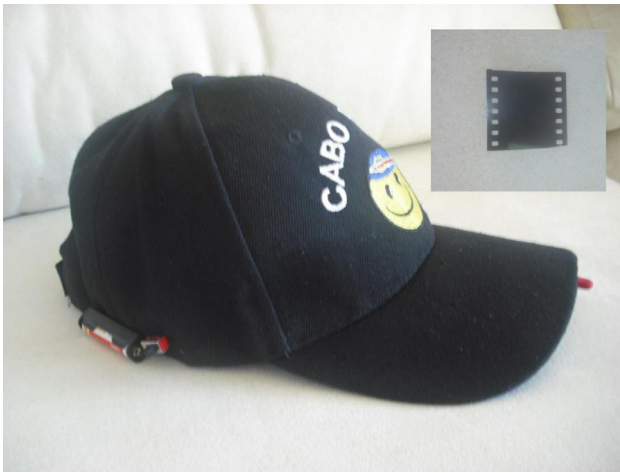
Fig. 20 It shows all the components of the MagiCap. At the front, we can observe the ir led, it is covered by a small piece of a red balloon (in order to dim the ir light). On the right, both the battery and the switch have been affixed. A piece of the negative film shown at the top right corner must be adhered to the laptop webcam
