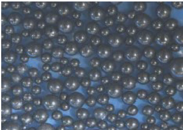
Fig. 3 ULW-1.05 ultralightweight proppant (Brannon et al. 2009)
