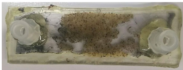
Fig. 1 Digital image of the micromodel (7.5 cm × 2.5 cm) used in this study. This image was captured after the flow experiment was terminated
