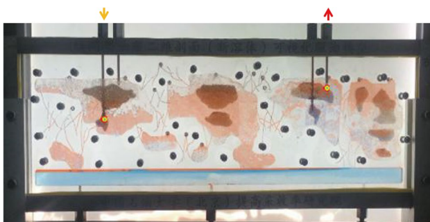
Fig. 9 Fluid distribution at the end of primary gas flooding when 70% of pore volume was filled in Scenario D
