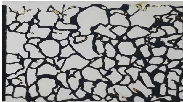
Fig. 8 Oil-saturated micromodel showing the remaining water (white color) after oil injection
