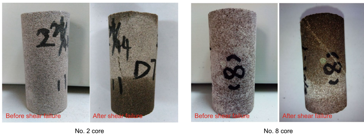
Fig. 1 Core samples before and after shear failure
